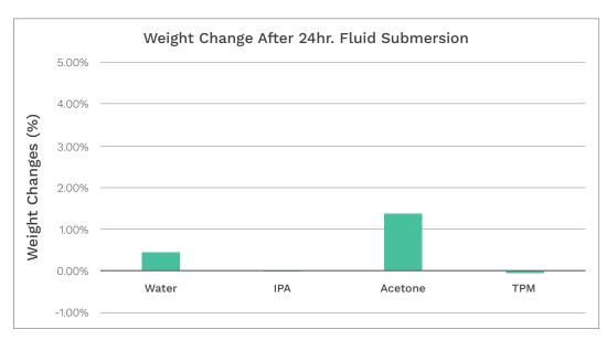
2" diameter discs (1/8" thickness) were 3D printed & post-processed, dried for 24 hours at 50°C, and submerged at room temperature conditions for 24 hours complying with ASTM D570 for water resistance and ASTM D543 for chemical resistance. Weight before and after submersion was measured and resulting percent changes were calculated.
