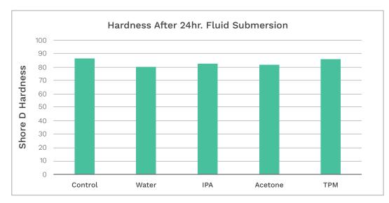
2" diameter discs (1/8" thickness) were 3D printed & post-processed, dried for 24 hours at 50°C, and submerged at room temperature conditions for 24 hours complying with ASTM D543 & ASTM D570. Resulting Shore D hardness was measured via ASTM D2240.
