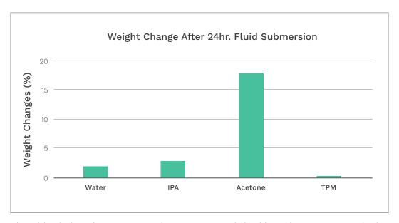
2" diameter discs (1/8" thickness) were 3D printed & post-processed, dried for 24 hours at 50°C, and submerged at room temperature conditions for 24 hours complying with ASTM D570 for water resistance and ASTM D543 for chemical resistance. Weight before and after submersion was measured & resulting percent changes were calculated.
